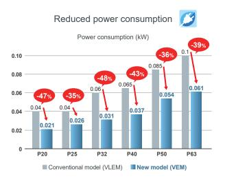
\*Measurement conditions (Power source: AC220-240V/50Hz, Fan speed: High) The unit consumes the same amount of power in both cooling and heating modes.
