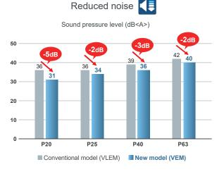
\*Measurement conditions (Measured point: 1.5m×1.5m, Power source: AC230V/50Hz) The sound pressure level is measured in an anechoic room.
