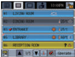
LIST screen Displays the operation status details of each group by group name.
