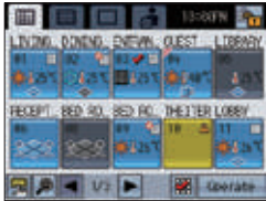
GRID (zoom in) screen Displays the operation status details of each group.
