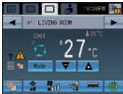
GROUP screen Displays the operation status details of each group. Sets group operations.
