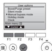
Setting method of the Manual bypass mode.
