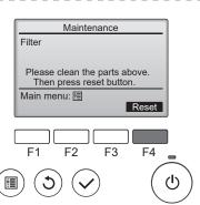
Press the F4 button to reset cleaning sign. See section 6 to clean the filters.
