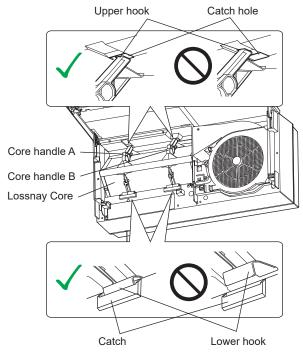
3) Check that the louver is closed and close the panel. (If the louver is open, the panel may get damaged.)
