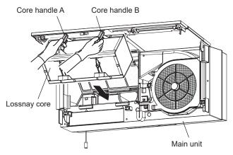
(2) Hook the lower hook of core handles A and B on the catch (1) then hook the upper hooks in the catch holes (2) as shown in the figure below.
