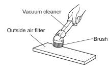
When the filter is heavily soiled, press and wash the filter with cold or warm water (40°C or less), and then air-dry the filter.
