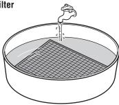
Do not use detergent. Also, do not scrub it. This may cause the platinum catalyst and activated charcoal filter to become damaged.
