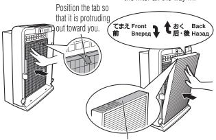
Do not push this surface downward. This may cause deformation.
