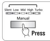
Each press changes the air volume, and the lamp for the selected air volume lights up.
