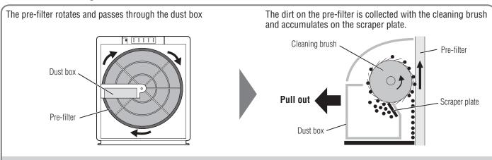
The dust accumulated on the scraper plate may gather together into a long belt-like shape that does not drop into the dust box. If the dust on the pre-filter is removed, the cleaning mechanism is working properly.
