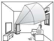
Air flow is controlled so that air is not blown directly at a person.
