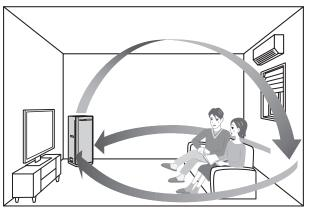
The air inlet and outlet are moved by the AUTO TURN which moves the main unit according to the person's location. The optimal air flow is created by the louvre in order to clean the area around the person.
