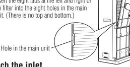
**5** Attach the inlet panel to the main unit.
