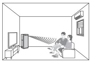
The i-see Sensor turns approx. 150 degrees in the left and right directions to detect the direction to a person's location.
