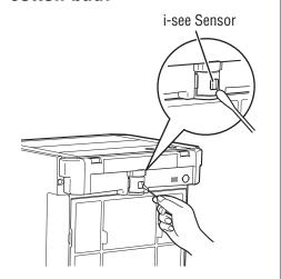
Do not wipe with water, alcohol, cleaning agent, etc. This may cause a malfunction. Do not use detergent, scouring powder, chemically-treated cleaning cloth, gasoline, benzene, thinner, etc. This may damage the main unit.
