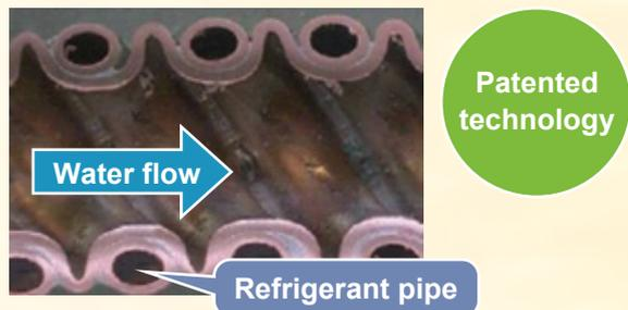
Using twist pipes as water pipes and running the refrigerant pipes along their grooves help increasing the heat-conductive area, allowing for better heat transfer.
